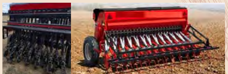
Photo n°46 Semoir direct VS semoir conventionnel
